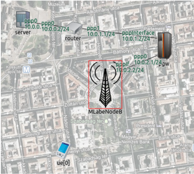
Figure 3. A screenshot of the simulation based on OMNeT++, the INET framework and simulte.
